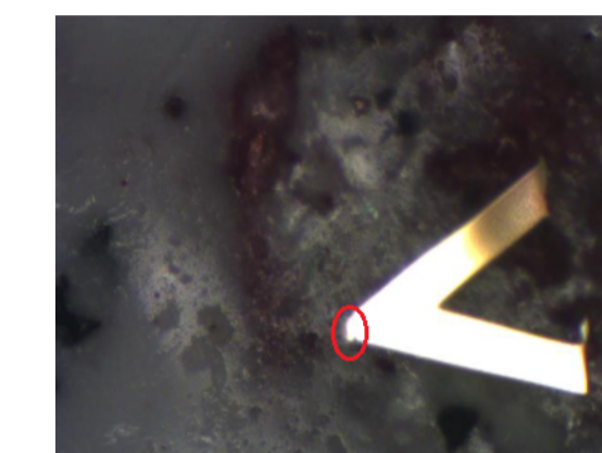
Figure 5: Cantilever and its rounded tip. Tip radius approx. 10nm
