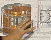
Fig. 1. 3D model of the in-vessel RMP coils and photograph of the physical coils.
