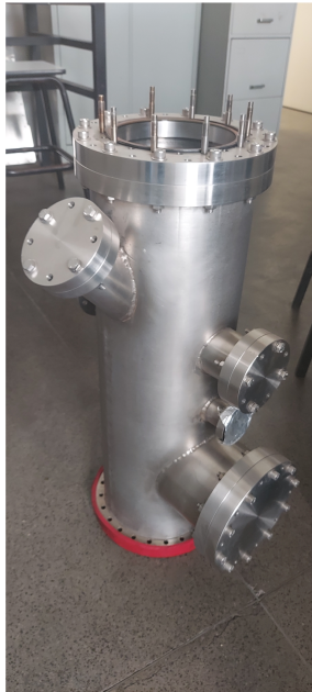
Figure 1: Picture of the hull of the tube
