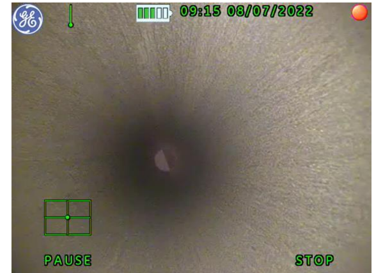
Endoscopic view of the TiZrV coated test pipe after the LP cycle
