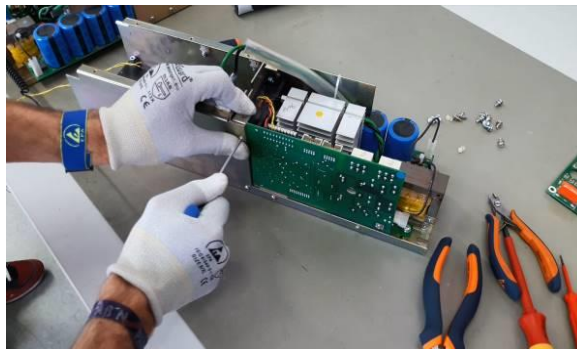
Family A PCO output power stages repair
