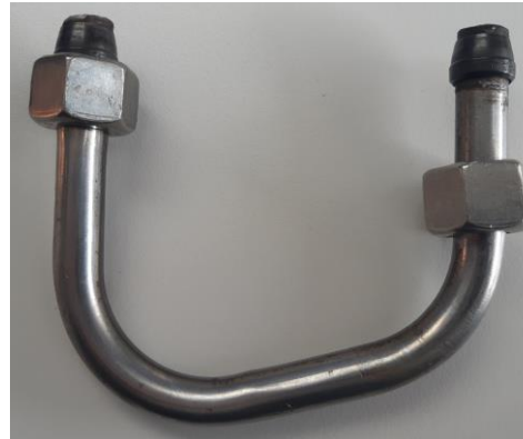
Family C4 clogged water pipe
