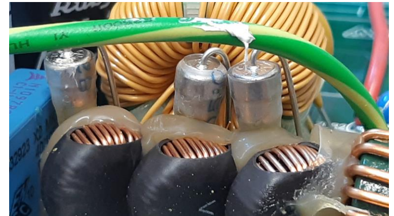
Broken Mean Well TDR-960-48
