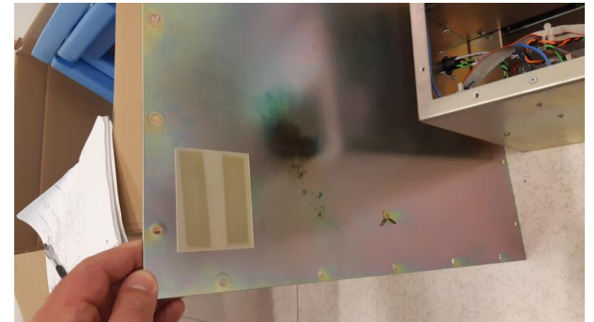
Family A2 PCO input power stage explosion
