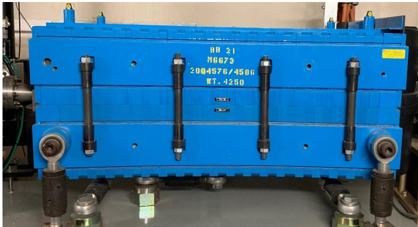
Booster Bend Dipole Magnet
