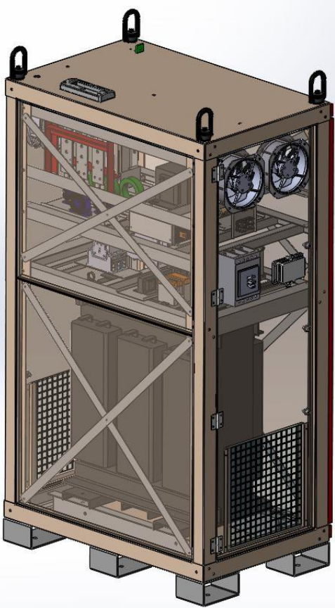
AC Input & Transformer Cabinet
