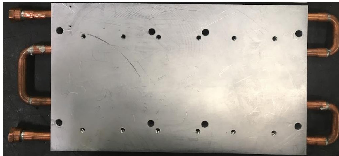
Existing Cold Plate Copper Tube OD=0.45"
