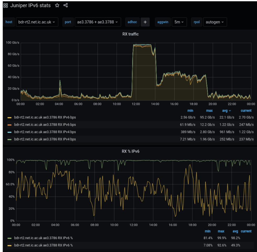
Figure 1 — Imperial monitoring shows the two-hour period where the 100G link was filled and where 100% of the LHCCONE traffic was IPv6.
