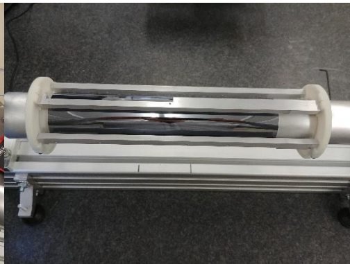
Support for gluing the longerons
