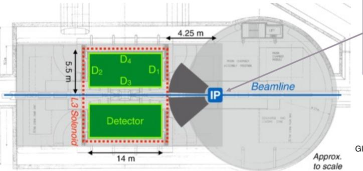
ALICE interaction point moved by 11.25 m outside magnet to allow LLPs to travel before decaying
