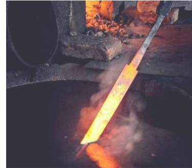
“Quenching” a rapid cooling process
