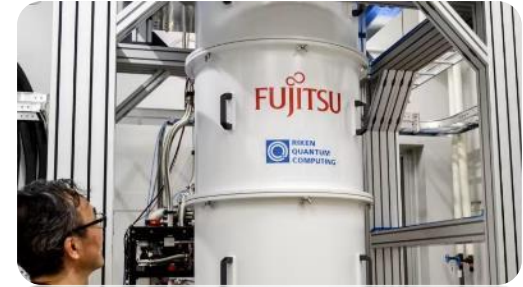
FUJITSU/RIKEN Quantum Computer 64 qubit superconducting gate-based
