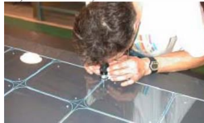
Scintillator tiles with wavelength shifting fibres
