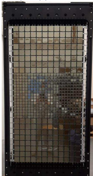
Multi-anode Photomultiplier Tubes for RICH upgrade (2022- ) (QE=45% @400nm)
