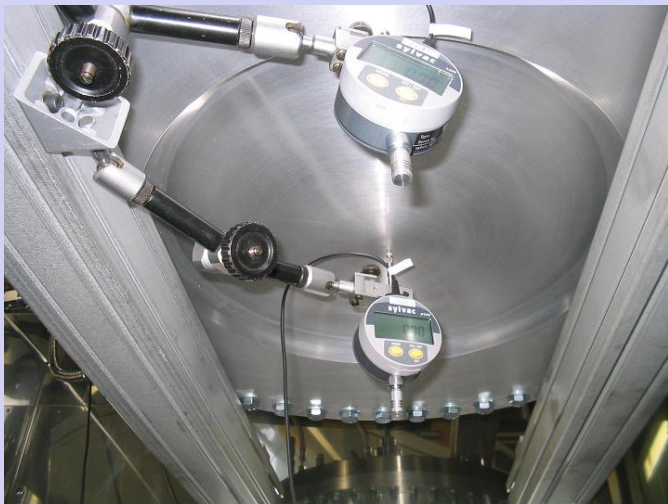
Pressure test (0 to 21.5 bar)
