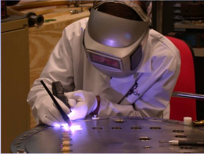
TIG welding of 20 HV 37pts feedthrough connectors and gas feedthroughs
