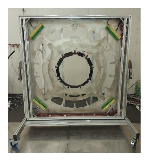
Ad-hoc design of "dummy module" to verify thermal path through <u>each individual insert</u>
