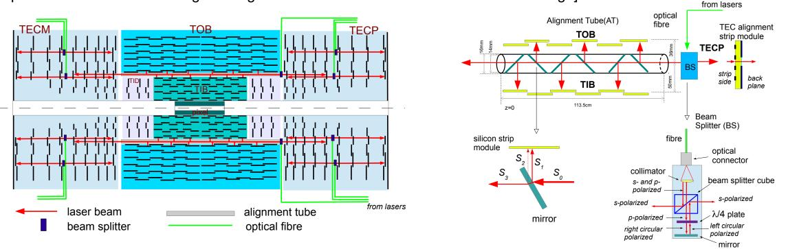
32 beams operate within the EndCaps, where special sensors were designed and produced, with a hole in the backplane metallization to let the light through
