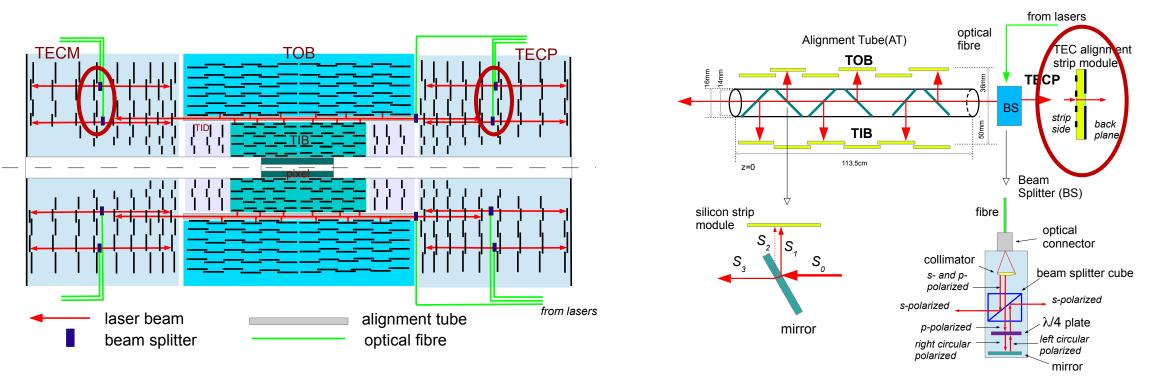
8 beams link some of the modules of the first Outer Barrel layer, with some of the module of the last Inner Barrel layer and some EndCap modules
