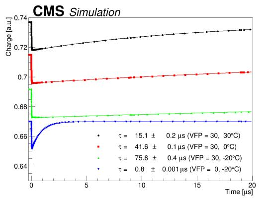
At the same time the operating temperature had been lowered, which increases the recovery time (This effect had been overlooked during the chip characterization)
