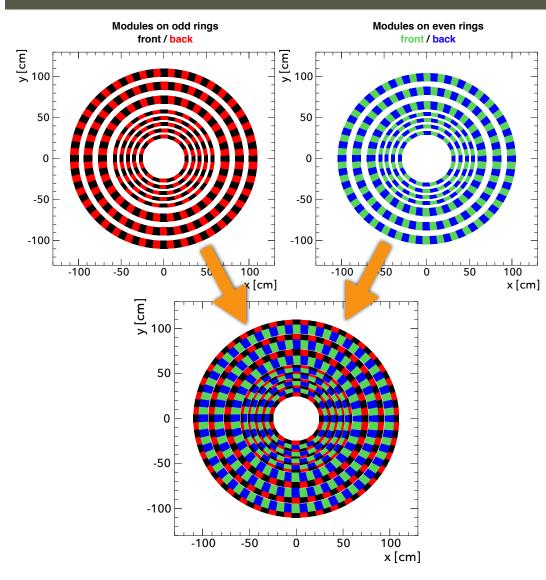
Use same modules as the in the barrels Strips are *not* pointing to the beam line
