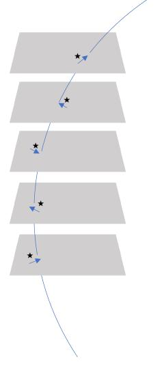
Connect hits collected in the different layers of the detector, identify trajectories of charged particles and measure their parameters
