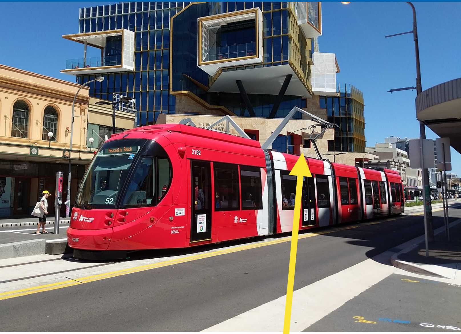
Battery charging at tram stop (Australia)
