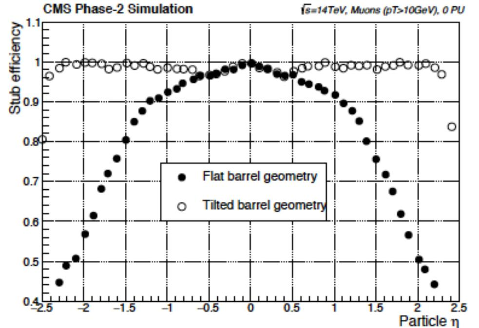
The stub acceptance at the edge of the layer would drop below 50%!
