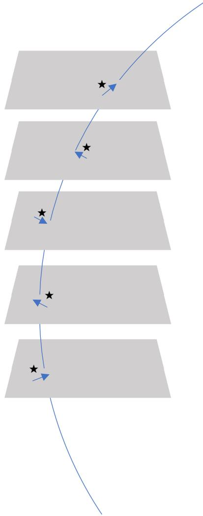
**Track reconstruction** also enables to determine the **precise position in space of all the modules**, well beyond the geometrical precision of the mechanical structures, by minimizing the **residuals**
