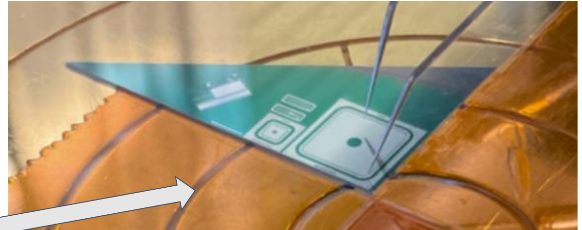
Example test structure diode
