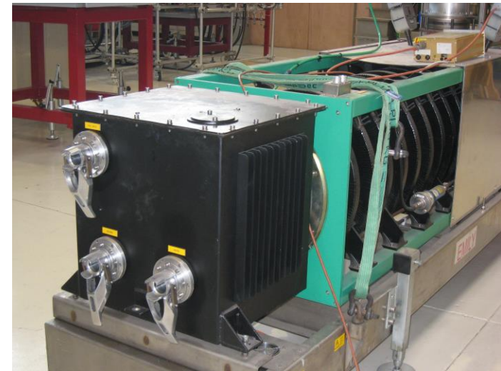
Klystron with oil tank and electrical terminals (anode power in oil tank)
