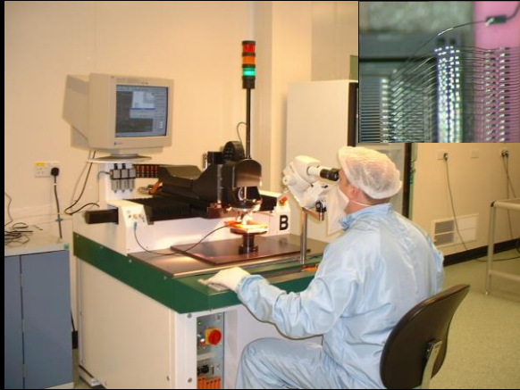
Module wire bonding (~5,000 bonds per module)
