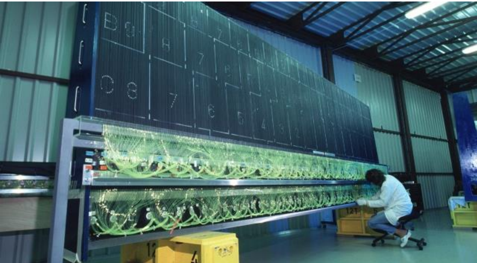
Instrumentation of the Tile Calorimeter barrel modules
