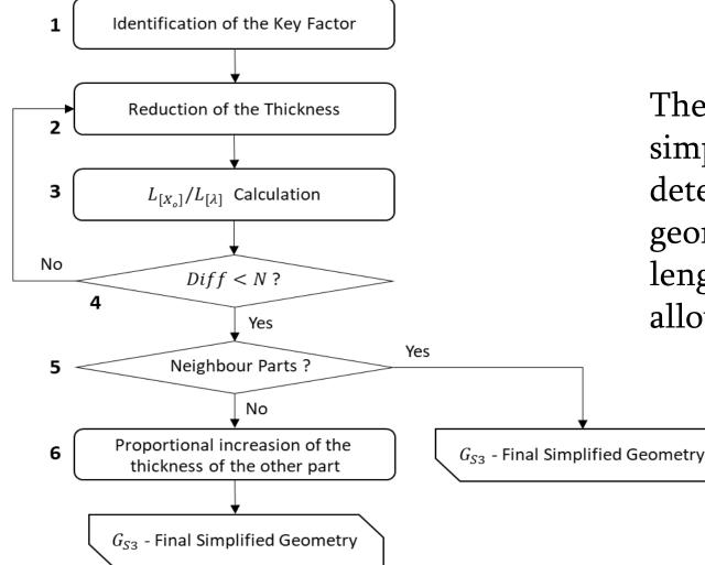
The general algorithm of simplification foresees the detection of regions in the geometry where the radiation length changes exceed the allowable value.
