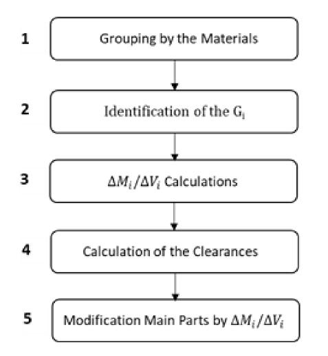
The purpose is to compensate for material loss after the  $\Pi_1$  and keep mass properties and volume of the initial, non-simplified geometry
