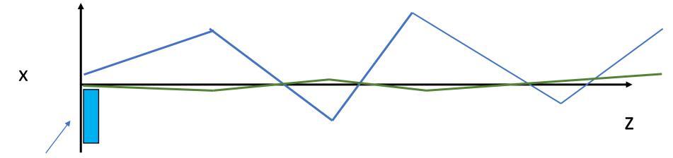
Orbit corrector creating a deflection. An orbit corrector is a dipole that is used to steer the beam
