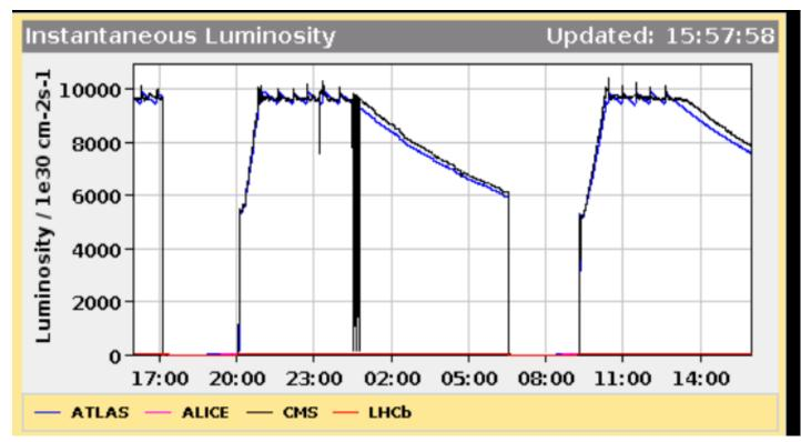
Screenshot from the 7<sup>th</sup> of May when I was on shift and CMS wanted to reduce the pileup slightly. Done by separating the beams slightly.
