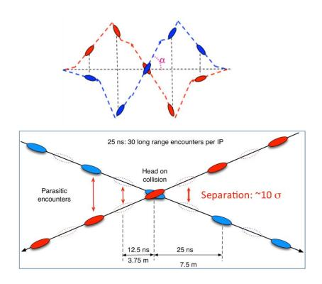
In case of a crossing angle one can calculate an approximative effective beam size following this formula
