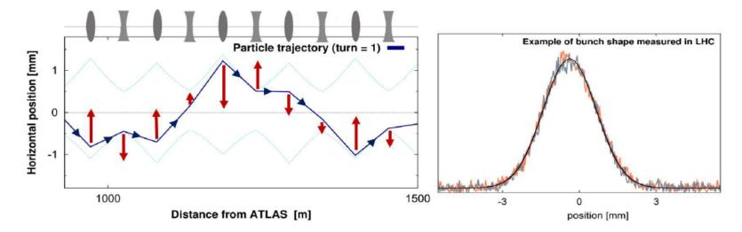
Particle motion about central closed-orbit described by Hill's equation:
