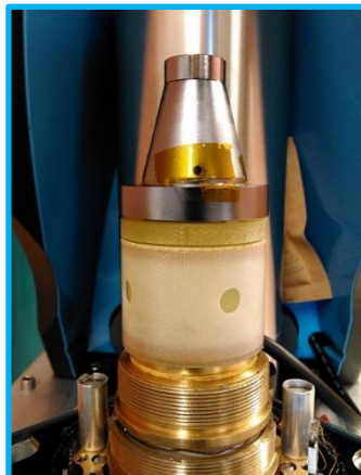
A JILA silicon Fabry-Perot cavity at 4 Kelvin frequency stability 6 \times 10^{-17} , drift < 5 \times 10^{-19}/s
