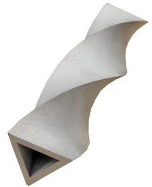
Fig.1. 3D printed twisted triangular waveguide
