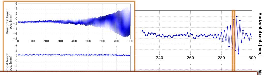
Horizontal coupled bunch instability observed during the 2015 scrubbing run in the SPS.
