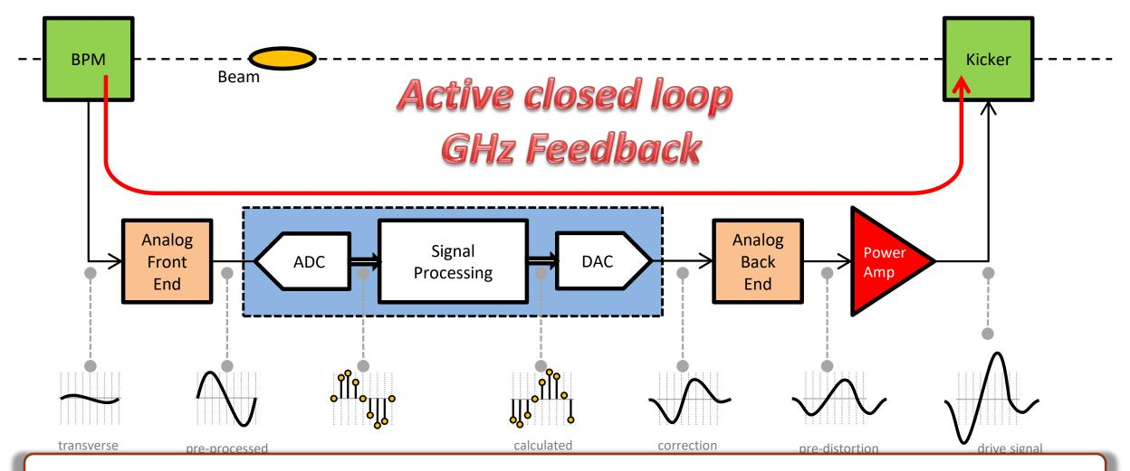
Simulations show that a wideband feedback system in principle can mitigate both TMCI and e-cloud driven instabilities.
