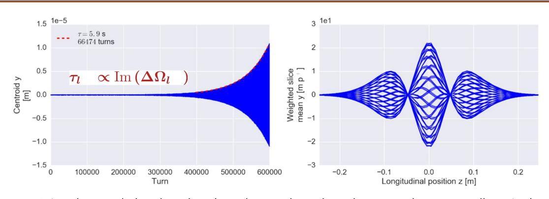
It is to be noted, that these bunch modes are always latently present, but not usually excited. It requires an **impedance as source of energy** together with **chromaticity to generate a synchronization** of the bunch motion with the wake fields kicks in order to **drive a given bunch mode into resonance**.
