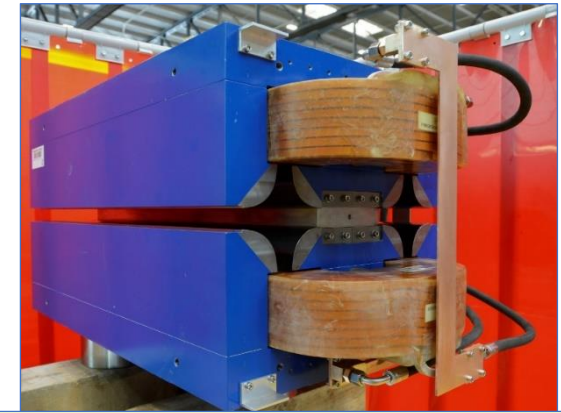
A. Milanese, Efficient twin aperture magnets for the future circular e^+/e^- collider, Phys. Rev. Accel. Beams 19, 112401 (2016)
