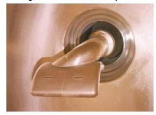
→ Coupler forms one half of capacitor with the gap
