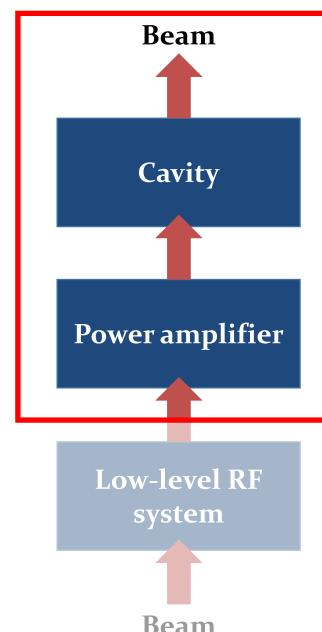
→ Convert RF power into longitudinal electric field
