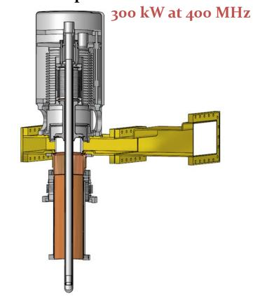
→ Coupler antenna transmits directly into the cavity
