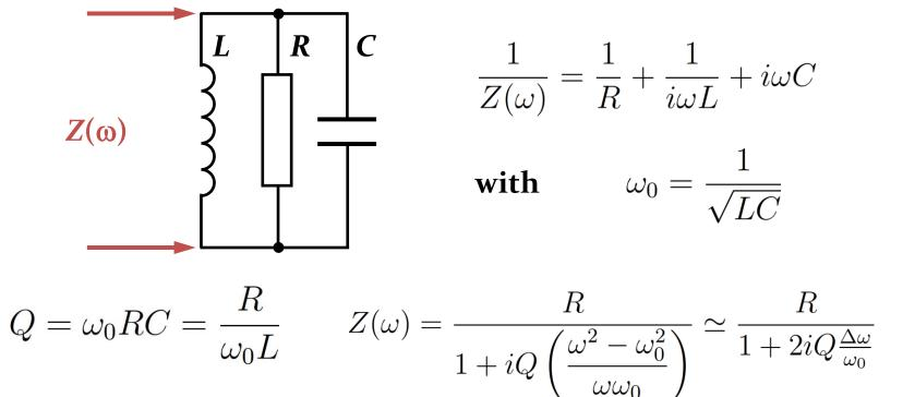
$\rightarrow$  Resonant circuit can also be described by R, R/Q,  $\omega_o$  or any other set of three parameters
