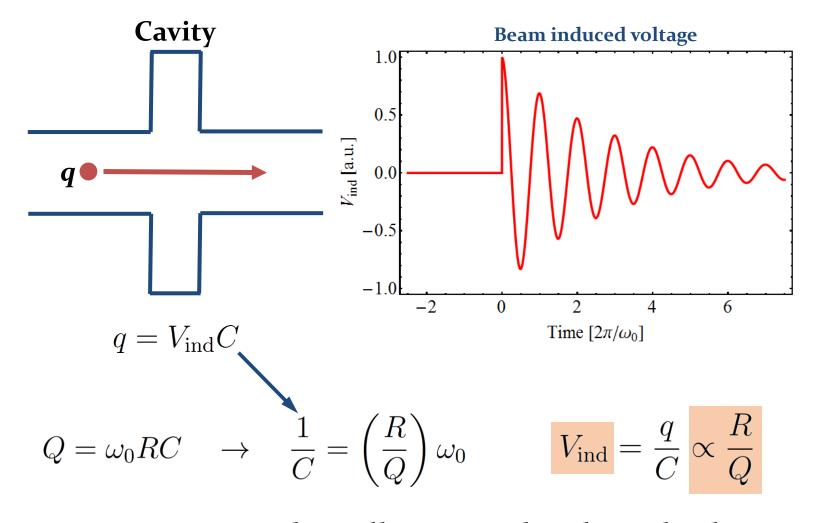
$\rightarrow$  Cavity geometry with small R/Q to reduce beam loading
