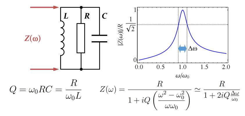
$\rightarrow$  Resonant circuit can also be described by R, R/Q,  $\omega_o$  or any other set of three parameters
