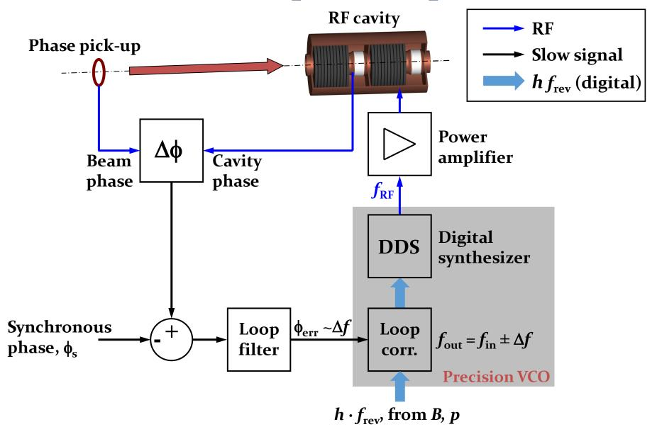
→ Phase-locked loop with beam phase as reference for RF system
