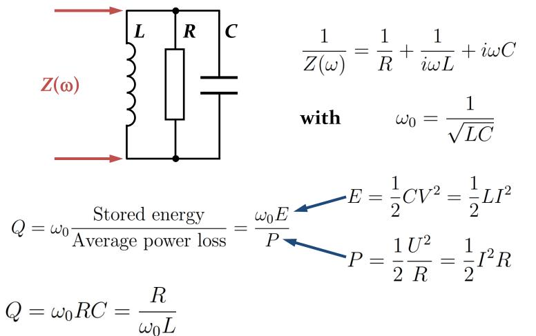
The resonance of a cavity can be understood as simple parallel resonant circuit described by R, L, C
