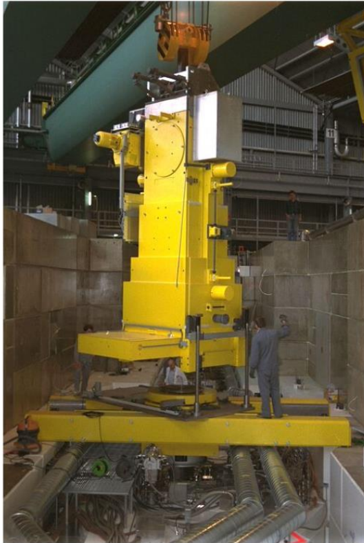
Figure 2.4-176: Radiation shielding bottle at PSI [65] to move activated parts to a hot cell. The whole plug is pulled into the bottle which is then transported with a crane.
