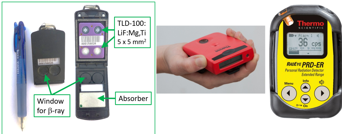
Fig. 16: Photos of several personal dosimeters: Left: pocket passive TLD dosimeter; middle: Geiger-Müller tube based active dosimeter; right: NaI(Tl) scintillator based active dosimeter.
