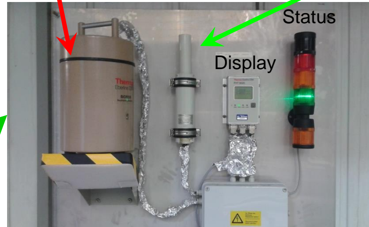
Moderated thermo-luminescence detector for passive n-detection
