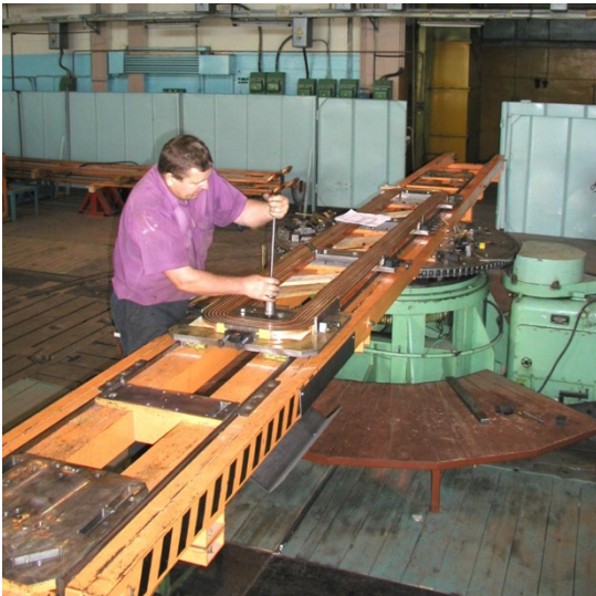
Dipoles racetrack coil
