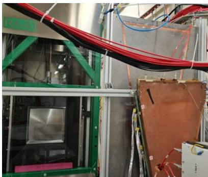
RPCs at tested at nominal rates at GIF++ (Nov.21)
