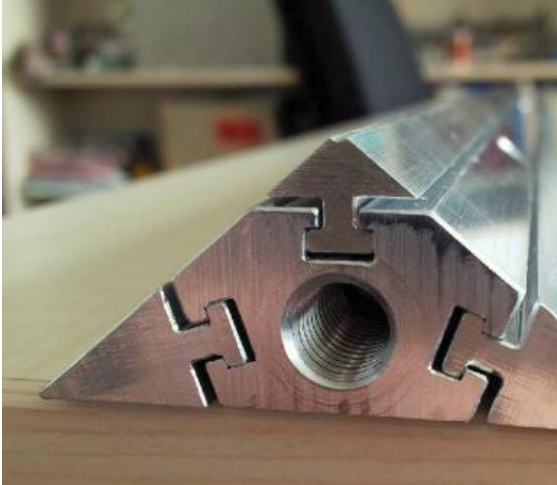
Hub for winding fibre on carbon fiber ladder with side pieces
