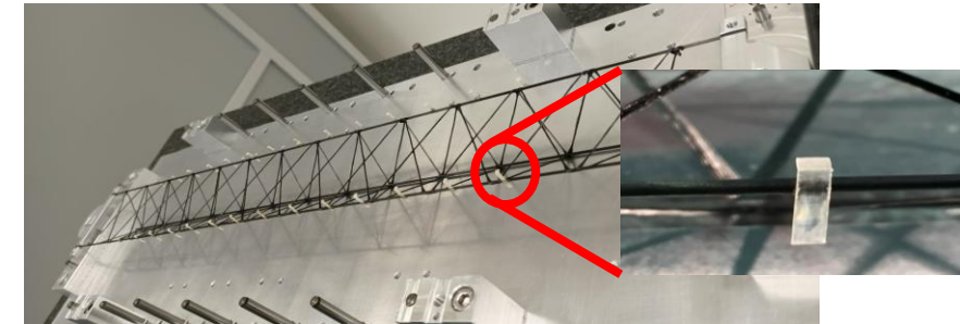
L-legs glued onto the ladder
