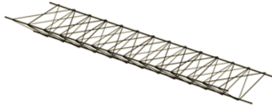
Light weight CF ladder – support structures for the modules
