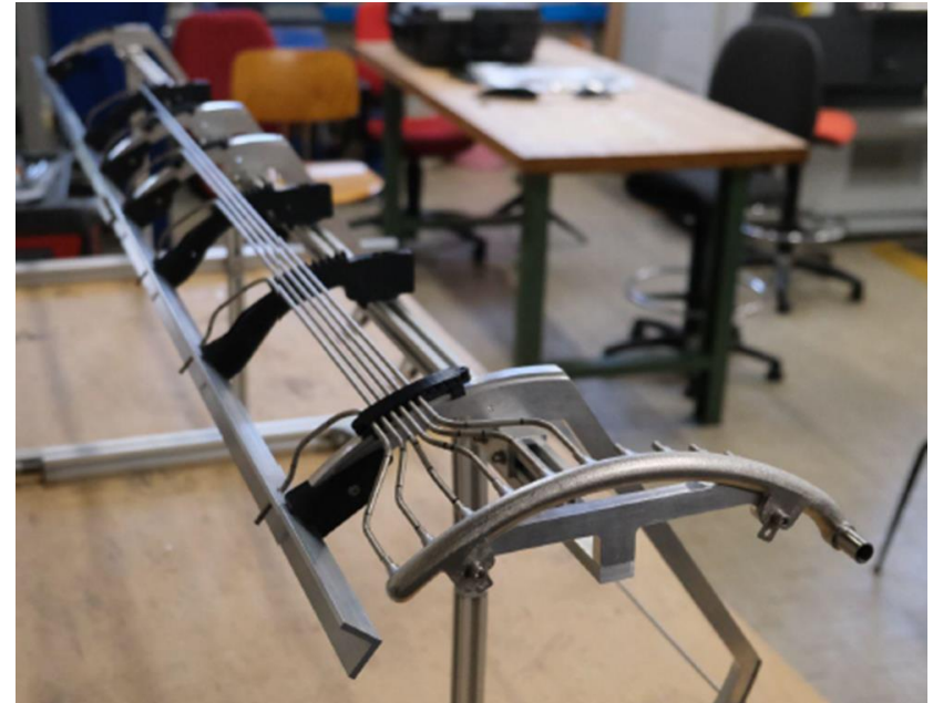
EC Pixel manifold (materials Ti6Al4V Grade 2 (pure Ti))
