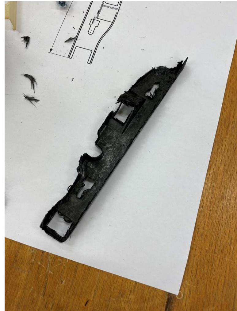
2 nd trial: too much material & improper closing
