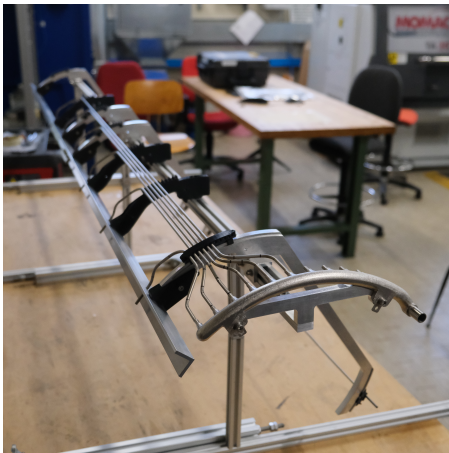
Prototype of Layer 2 exhaust line and manifold on integration tool
