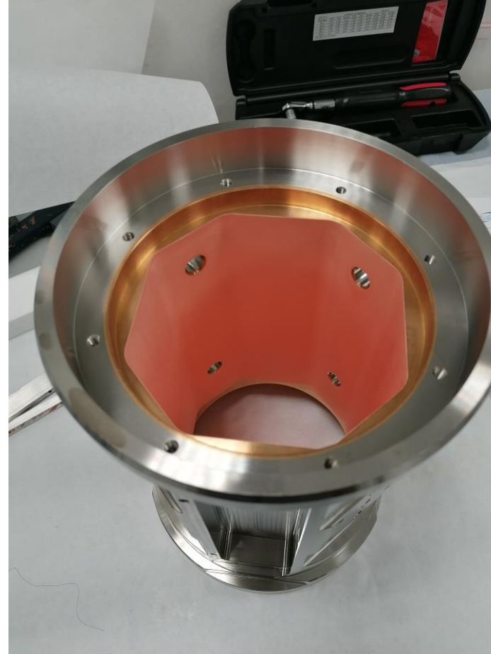
Gold and copper plating steps of LHC BPMs
