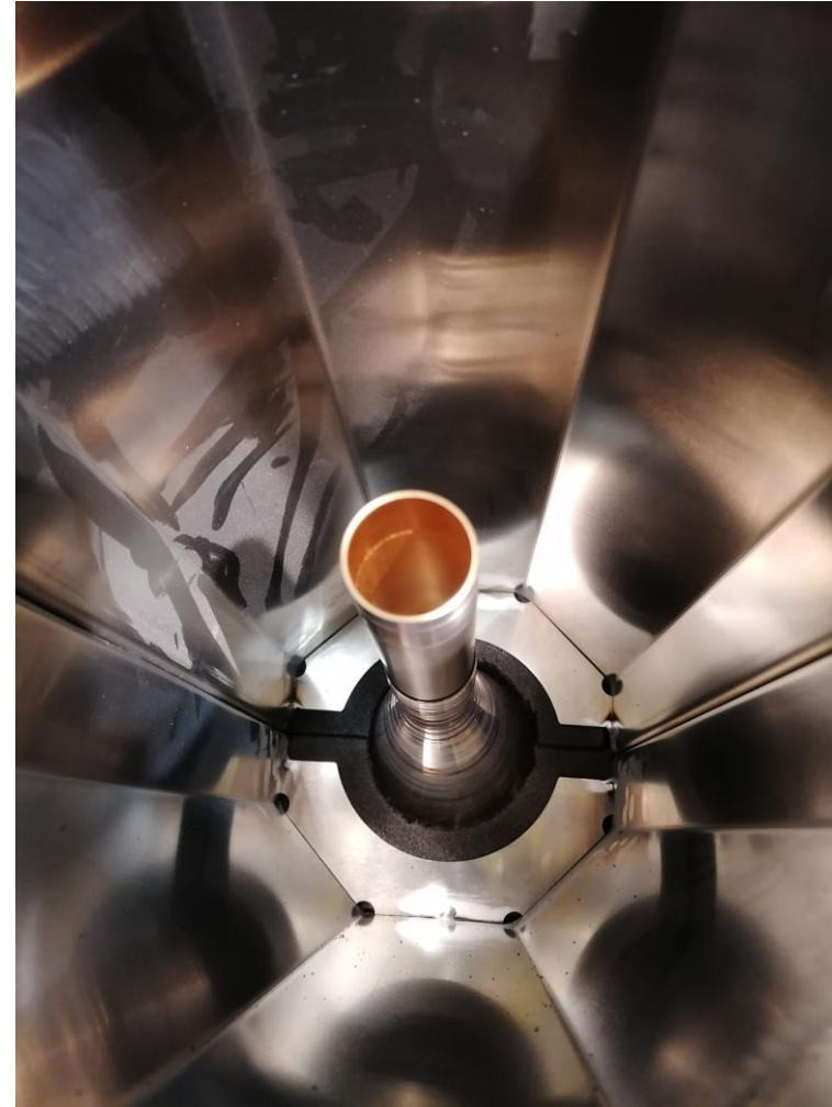
Gold plating of Kovar edge of the glass assembly for the FLOTUS experiment (CLOUD)
