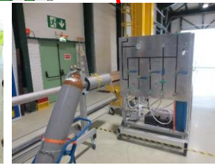
Pressure test of cooling tubes
