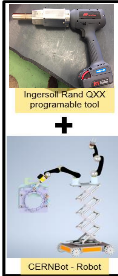
Programmable torque, angle, speed etc. through cable or Wi-Fi
