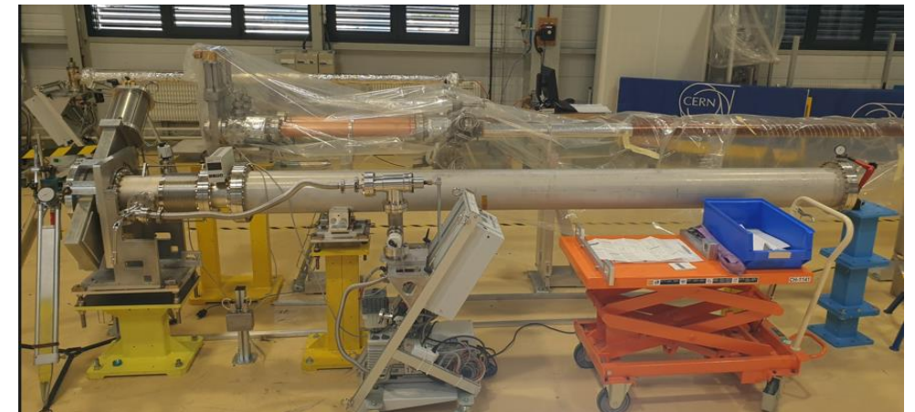
Deformation testing of vacuum supports in B113
