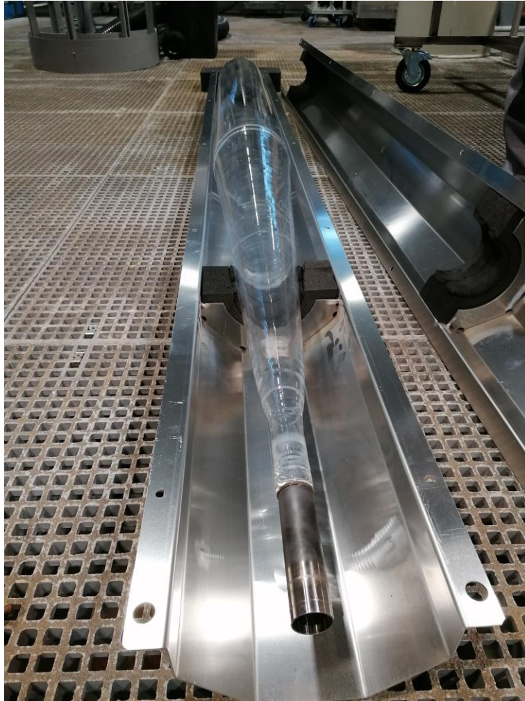
Gold plating of Kovar edge of the glass assembly for the FLOTUS experiment (CLOUD)
