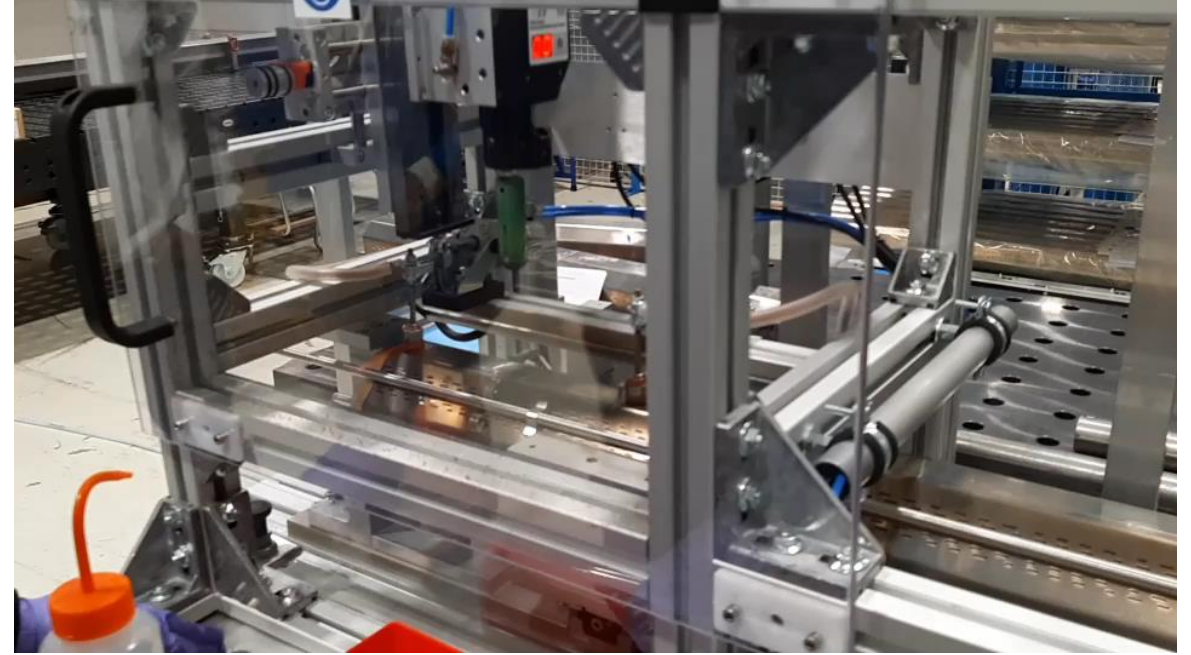
Stud welding on Q2 pre-series
