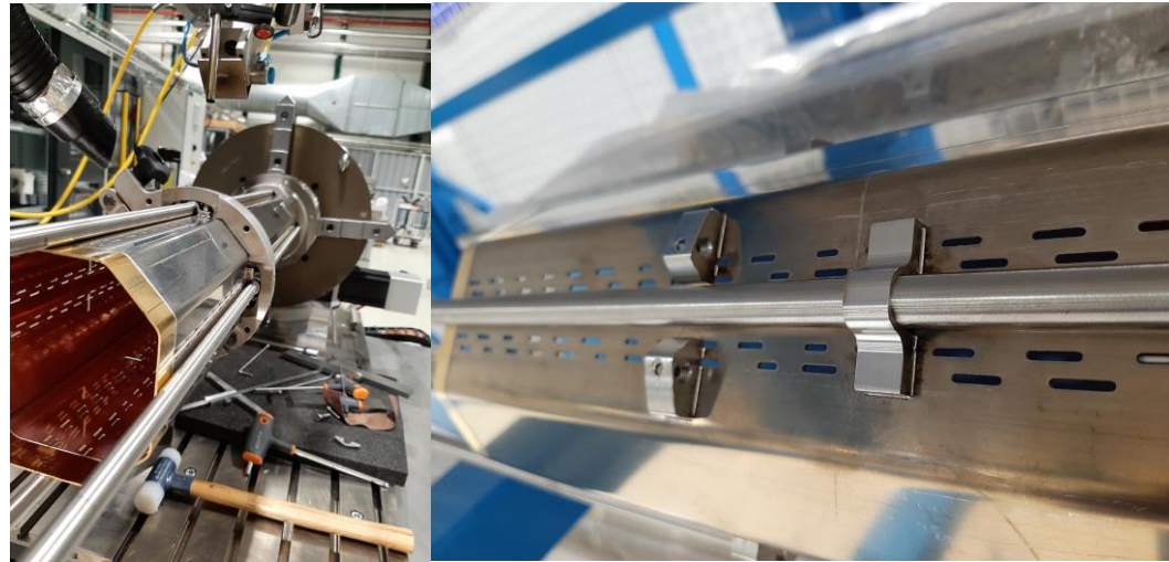
Welding of the contact rings, cooling tube supports and fixed points, completed
