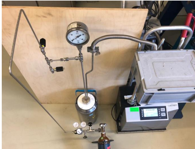
Sample and pressure cycling test set-up
