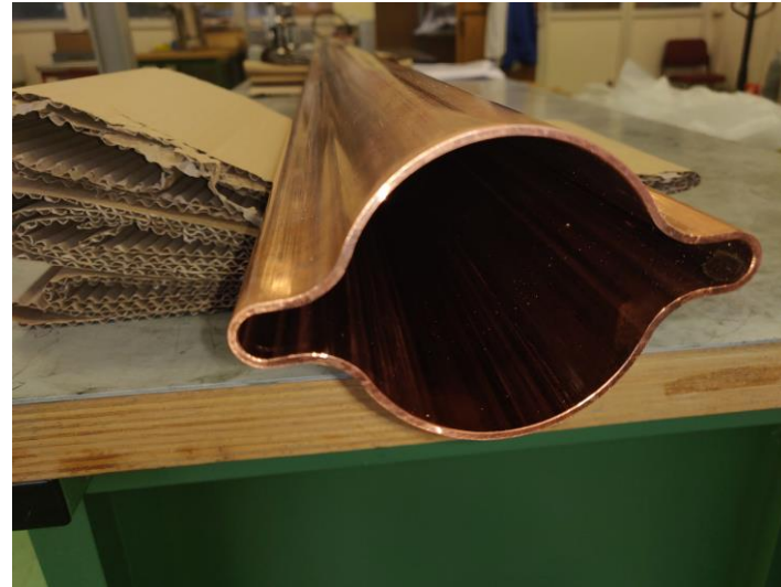
Cold extruded chamber in C10200, 2 mm uniform thickness
