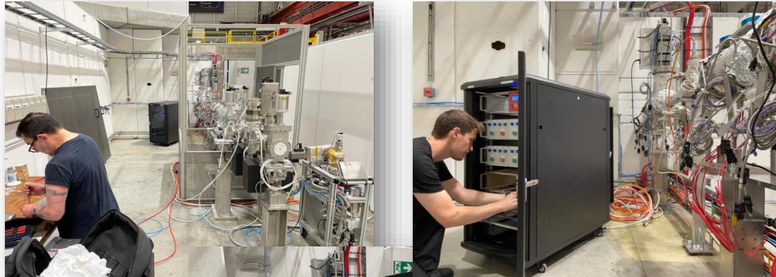
Local vacuum controls rack
