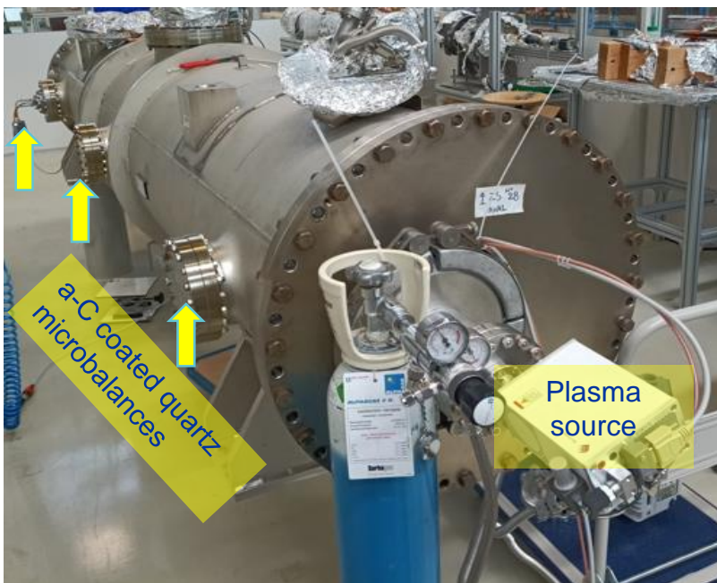
ZS tank D=600mm L=3500mm
