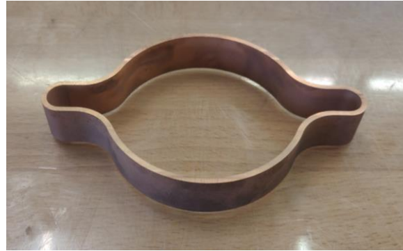
Short chamber profile made by wire-cutting (Erosion Discharge Machining)
