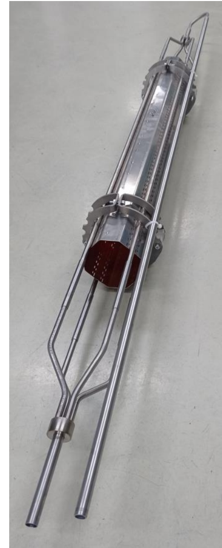
Model of the beam screen for cold leak/pressure test
