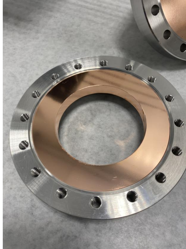
Copper plated flange before Nb coating
