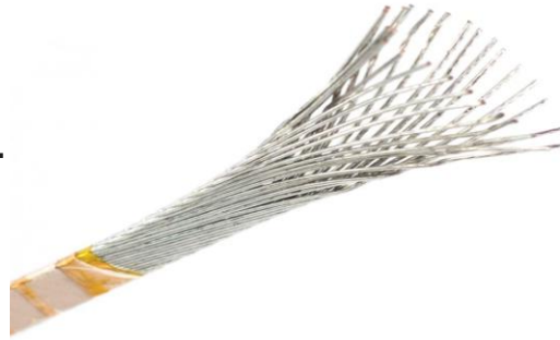
Rutherford cable coated with SnAg
