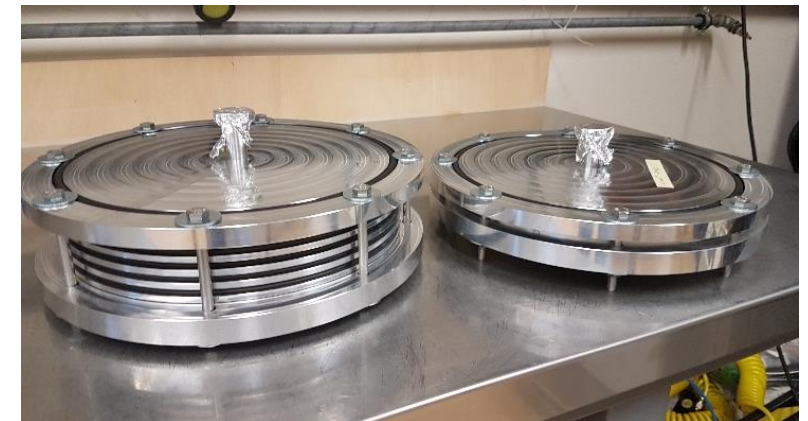
Irradiation campaign of elastomer seals
