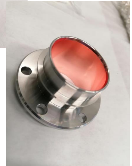
RF contacts inner CRAB line (copper plating on stainless steel)
