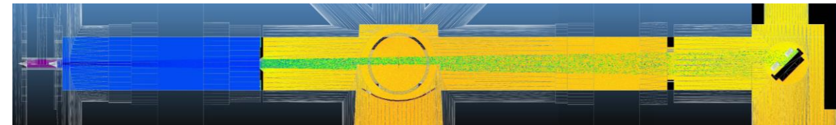
Pressure in vessel & particle density due to gas jet
