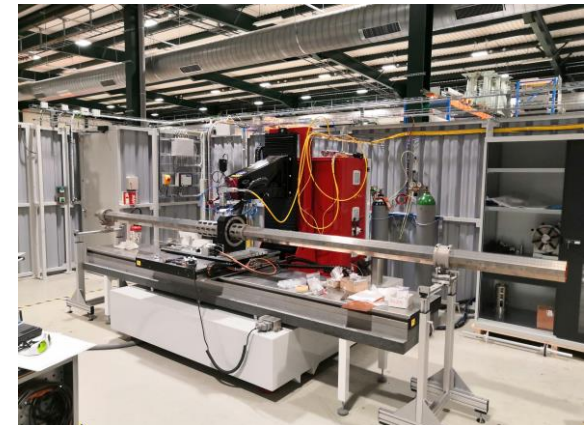
Butt welding of the beam screen segments
