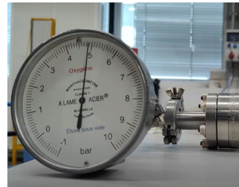
1 \mu m 6x6mm Si 2 N 3 window \rightarrow \approx 5 bar pressure
