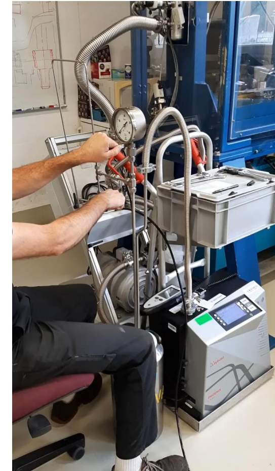
Pressure cycling at room temperature and 77K (3000 + 3000 cycles without sign of leak)
