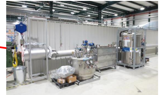
Cold leak/pressure test
