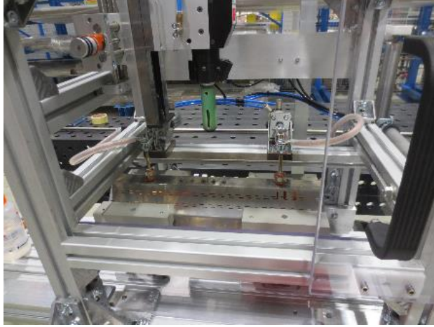
Completion of the dedicated bench for the stud welding of the absorber pin supports
