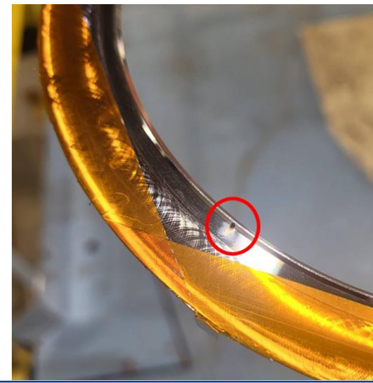
Spark PSB seal (faulty RF bypass)
