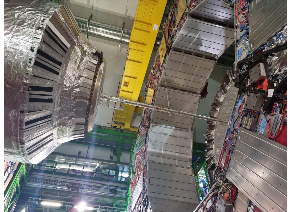
Opening of the YB+2 central segment during LS2
