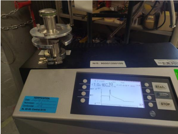
Helium leak testing. Tool developed to test: - Deposit + Substrate - Deposit only - Interface
