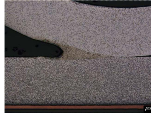
Metallography for the cooling tube weld qualification
