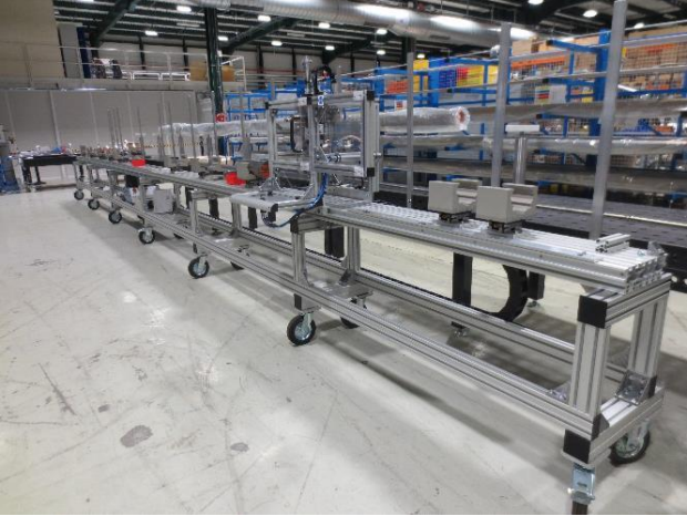
Completion of the dedicated bench for the stud welding of the absorber pin supports
