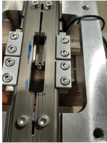
Completion of the dedicated bench for the stud welding of the absorber pin supports
