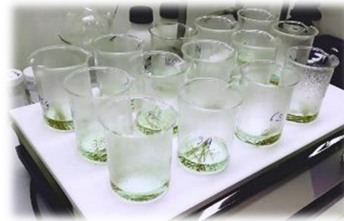
Acidic solution etching of SnAg coating
