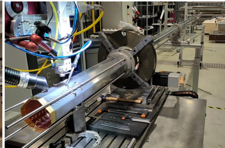
Welding of the contact rings, cooling tube supports and fixed points, completed
