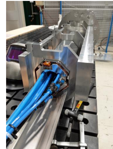
Micro-TIG tack welding, completed
