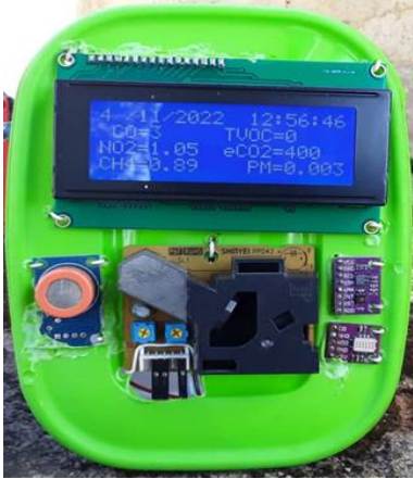
Zigbee based IoT device (PM2.5, CO, CO2, NO2, VOC and CH4)
