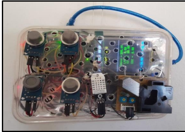
GPRS based IoT device (CO, CO2, PM2.5, GPL and Smoke)
