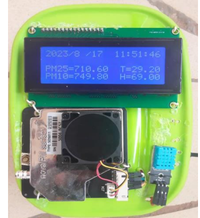
IoT device based on Thingspeak cloud (PM2.5, PM10)
