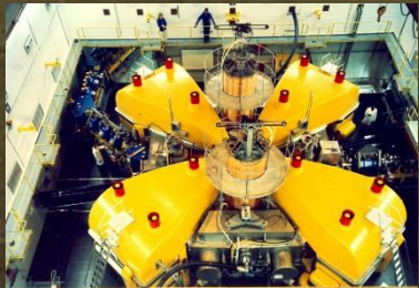
K200 Separated Sector Cyclotron (SSC)
