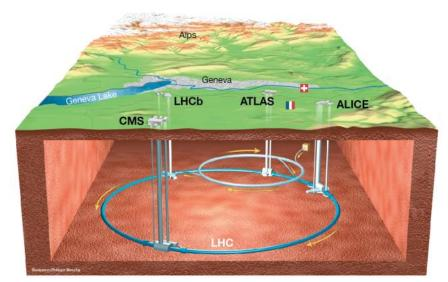
The two beams cross at four collision points which are the locations of the four major experiments of the LHC:
