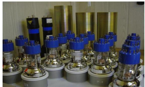
Fig.2. Stilbene modules attached with 3" PMT.
