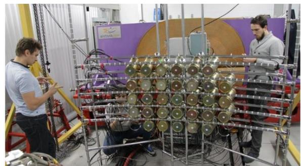
Fig.4. The experimental stilbene detectors being implemented at ACCULINNA-2.
