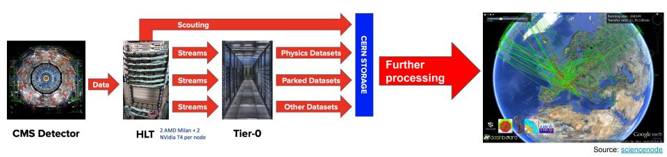
The Tier-O processes the data files and outputs RAW and other specialized streams data to CERN storage, divided into "Primary Datasets" (PDs), e.g. dimuon, e-gamma, JetMET.
