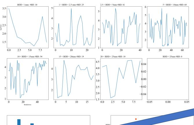
Here, I take the breakdowns that have less than 1mm distance (upper left) and plot the time difference they had (y in log). Second plot have the breakdowns between 1 and 2.5mm etc. (indicated above the plots).
