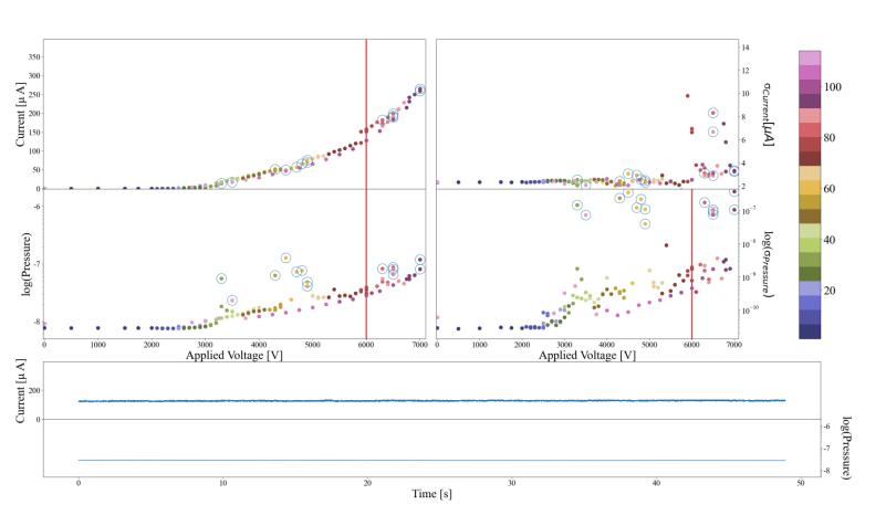
Each dot in the dataset represents a measurement. A breakdown in that run is represented with a blue circle. The red line indicates which measurement we are on and the applied voltage. In addition, the pressure and current áre shown in real time underneath, as each measurement lasts 50seconds.
