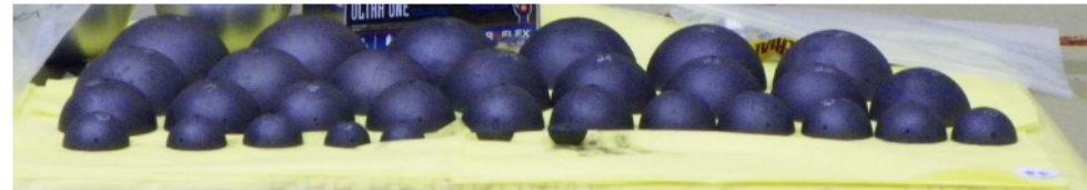
Highly-enriched uranium shells
