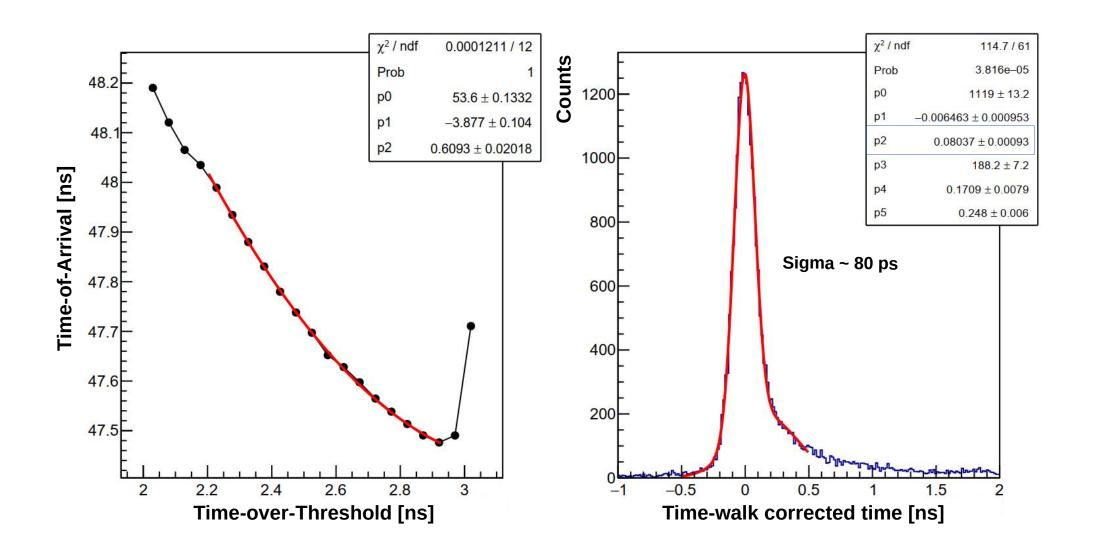
**<u>Timing resolution</u>** with LAPPD and PETsys: (left) distribution of time-of-arrival vs. time-over-threshold (proportional to signal amplitude), clearly showing time-walk effect, with the fit used for time-walk correction; (right) single photon timing resolution with **sigma around 80 ps** is obtained with after time-walk correction.
