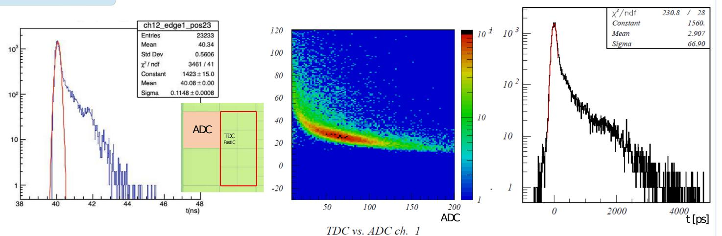
A single channel the size of 1/2" was illuminated at the center with a picosecond laser pulses. We measured the timing spread between the laser trigger and time-of-arrival (ToA) to be **<u>115 ps without time walk correction</u>** (left). While signal was too short for ToT detection, we used induced signal on the neighboring pad, measured by VME ADC, for time-walk correction (middle). After time-walk correction the timing spread of the prompt signal was ~ 70 ps (right).
