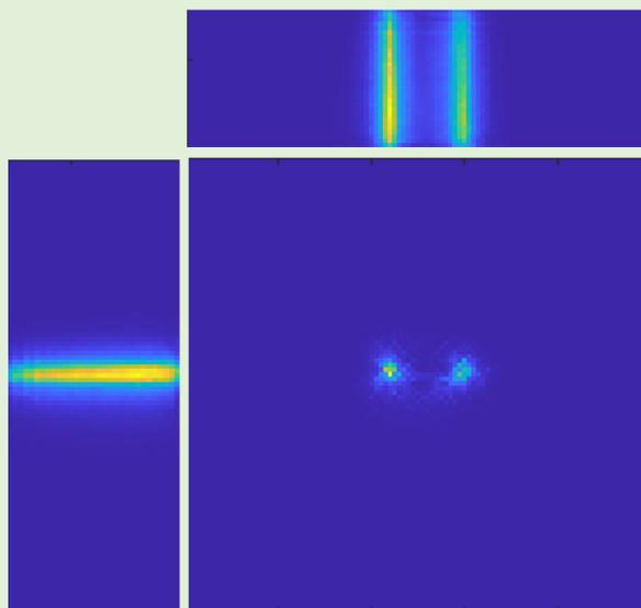
Figure 4: Reconstructed image with the data that corresponds to events in which both gamma-rays scattered with the polar scattering angle  $82^\circ \pm 10^\circ$ , with azimuthal angle difference of  $90^\circ \pm 20^\circ$  (preliminary).
