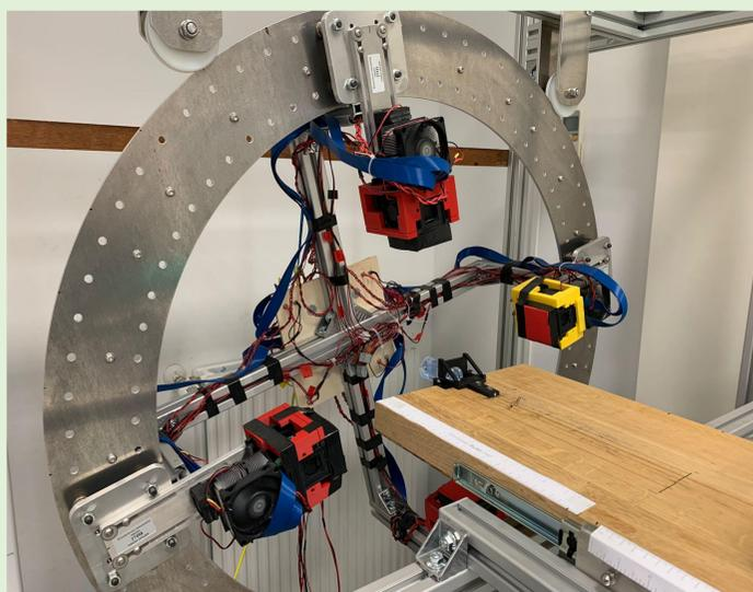
Figure 1: The novel PET demonstrator device. Detector modules based on the single-layer Compton polarimeters mounted on a rotating gantry [5, 7, 8, 9].
