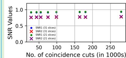
Figure 7: SNR values of images with the difference of azimuthal scattering angle  $90^\circ \pm 20^\circ$  and polar angle  $70^\circ \pm 10^\circ$  vs. number of reconstructed coincidences per position, calculated before and after the removal of the top and bottom 5 slices (preliminary).
