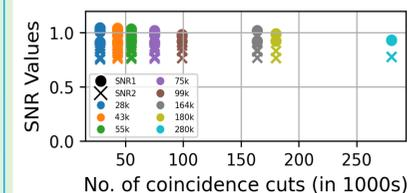
Figure 5: SNR values of all the reconstructed images vs. number of reconstructed coincidences per position (preliminary).
