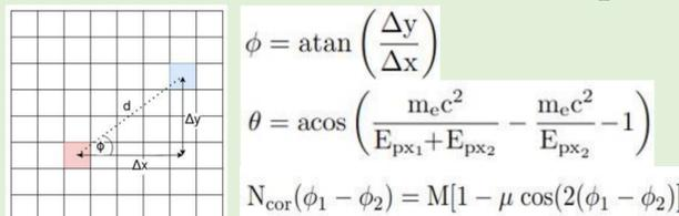
Figure 2: Polarized gamma-ray Compton scatters in one pixel of the detector and gets absorbed in another. The Compton angles are reconstructed from the equations.
