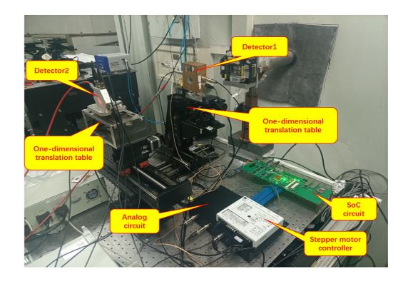
Since the SAPS has not been built yet, the feedback control system has been evaluated and tested in the Macromolecular Crystallography Beamline 1W2B at BSRF. The testing equipment and testing platform are presented in left Figure:
