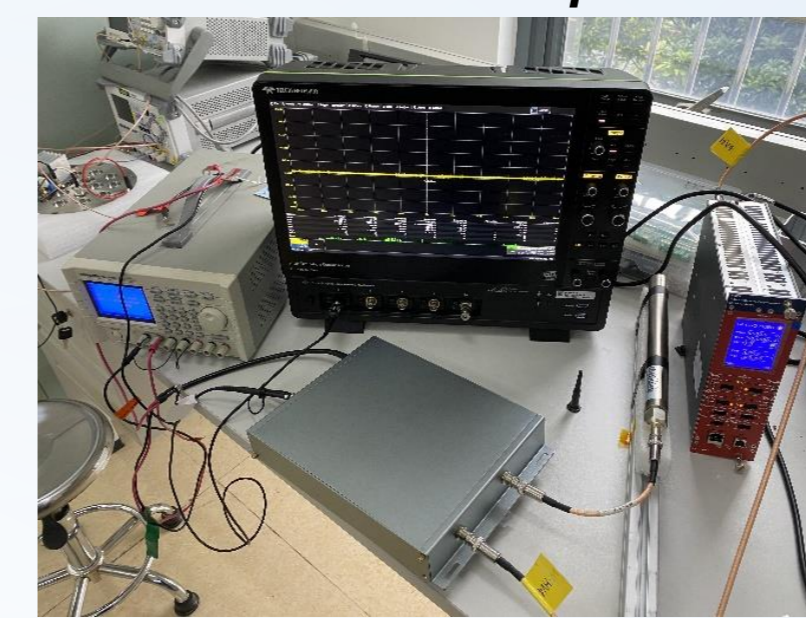
HEROCV1 Chip Connected to the Detector - Real-world Image (Left); Neutron Source Test Set-up (Middle); Neutron Signal Output Waveform through ASIC Shown on Oscilloscope (Right)
