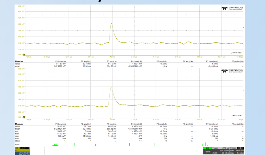
HEROCV1 Chip Connected to the Detector - Real-world Image (Left); Neutron Source Test Set-up (Middle); Neutron Signal Output Waveform through ASIC Shown on Oscilloscope (Right)
